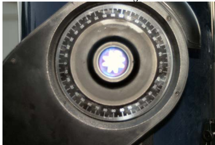
Illustration 5 - Setting the declination circle to observer's latitude
