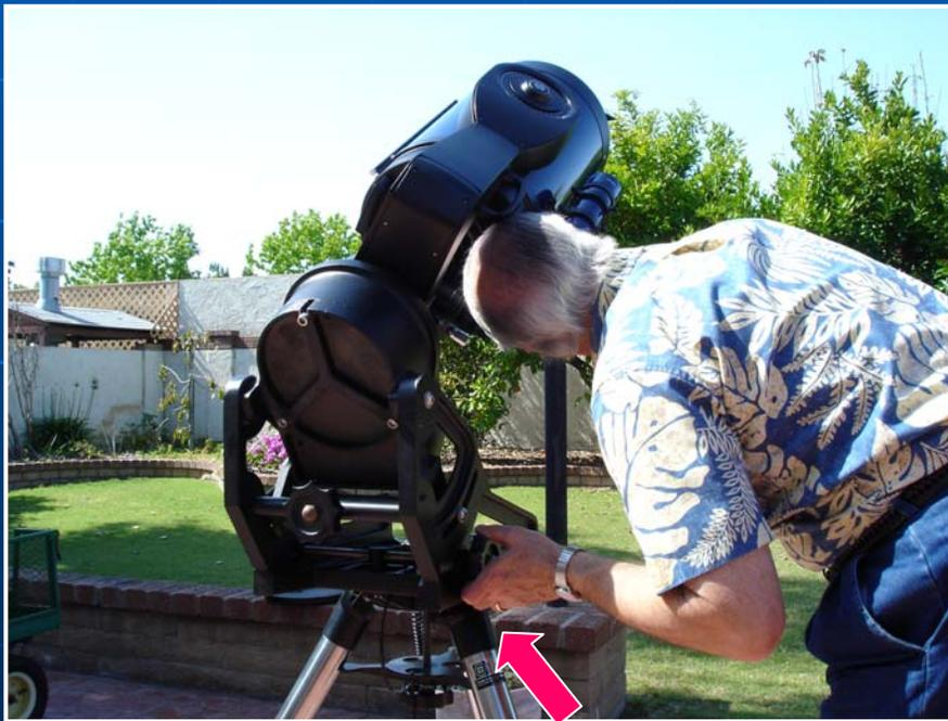
Manual Azimuth adjustment
